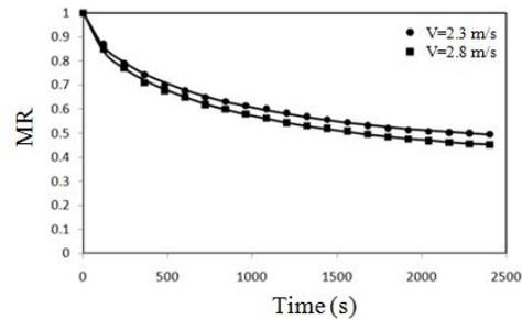
**Fig. 4.** Effect of superficial fluidization velocity (T: 50 °C, W: 1.32 kg).
