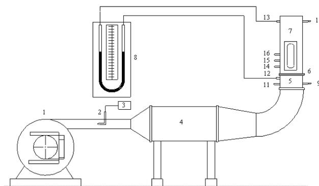
**Fig. 1.** Schematic diagram of experimental setup (1. Blower; 2. Pitot tube; 3. Differential pressure transmitter; 4. Electrical heater; 5. Air plenum chamber; 6. Distributor plate; 7. Dryer chamber; 8. U-tube manometer; 9-10. Relative plenum humidity sensors; 11. Temperature control sensor; 12-13. Pressure recording taps; 14-15-16. Bed temperature distribution sensors).
