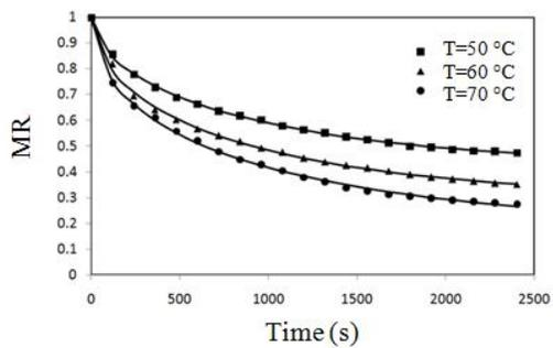
**Fig. 3.** Effect of temperature of drying air (V: 2.5 m/s, W: 1.32kg).
