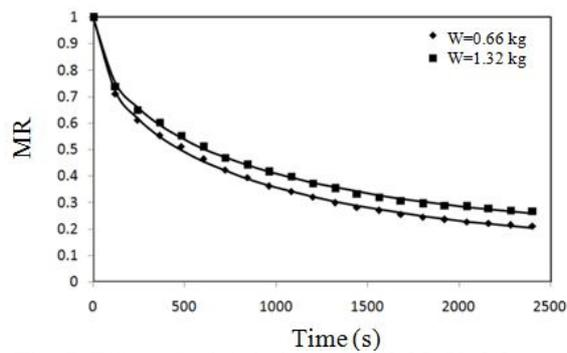
**Fig. 5.** Effect of solids holdup (T: 70 °C, V: 2.8 m/s).
